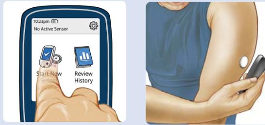
Touch **Start New Sensor**. Hold Reader within 1.5 inches (4 cm) of Sensor to scan it.
